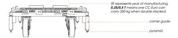
Non-functional bases can be handed in at a CC depot or partner depot for repair and exchanged for functional bases.
